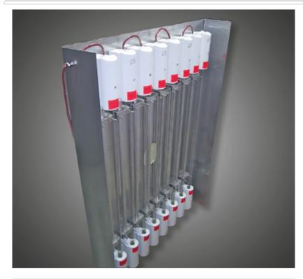
The UV-C moisture-proof fixture, which complies with protection class IP 65, has been specially developed for use in particularly damp and dusty environments. 253.7 nm UV-C radiation is used to reduce the number of germs. This wavelength has a lethal effect on microorganisms such as bacteria, moulds yeasts and viruses.
