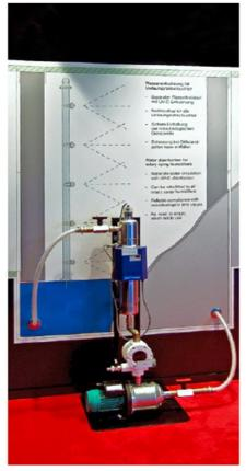
Air in HVAC systems is often humidified using rotary spray humidifiers. The excellent humidification effect is set against an increased microbial hygiene risk. This is why the German standardVDI 6022 "Hygienic requirements for ventilating and air
